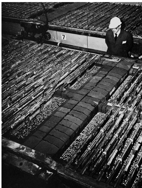
ALLPLAS ball blankets reduce moisture absorption by sulphuric acid solutions. Conversely, reduced acid mist generation cuts plant maintenance costs while improving working conditions.
