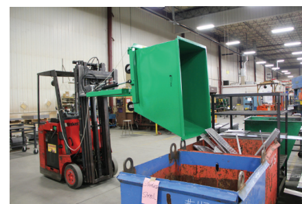
Step 3: Transport Mobile Hopper to dumping location and empty. When finished, lower completely to floor. Release Mobile Hopper from Fork Lift Attachment by easily pulling on the attached cord.
